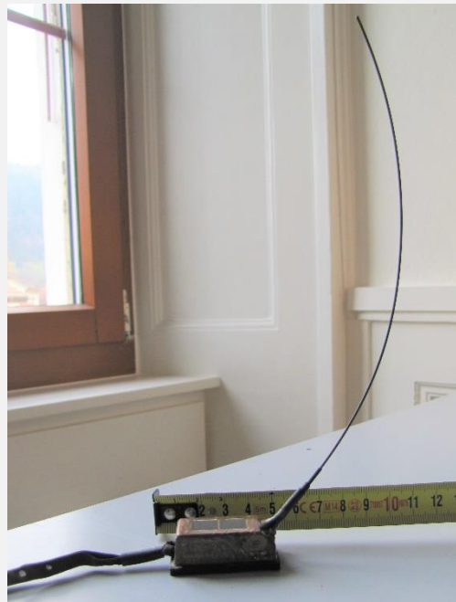
Figure 7: balise Argos avant la pose.
